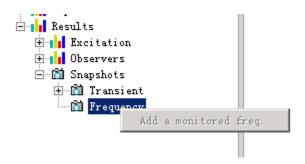
Note: in normal state, the freq. snapshot definition is disabled, you need to switch to "showing snapshot" mode to enable it.
