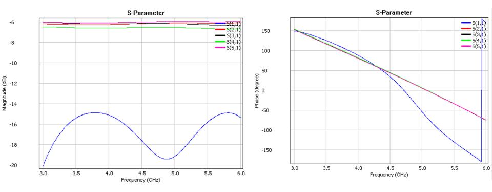
S11 is less than -15dB in a wide band and the phase difference of the four outputs is less than 1.5 degrees
