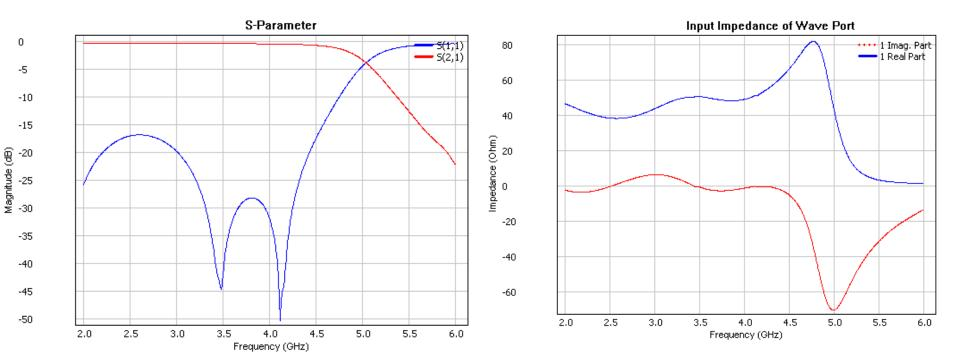
S11 is less than -30dB near 4GHz and the input impedance is near 50  $\Omega$ .
